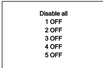
6. Turn the Dial to choose between **<Disable all>** which turns off all alarms or any of the 5 alarms. Press the select button to set the alarm that you want to activate. Below is an example to set Alarm 1. Choose **< 1 Off 12:00 AM >**
